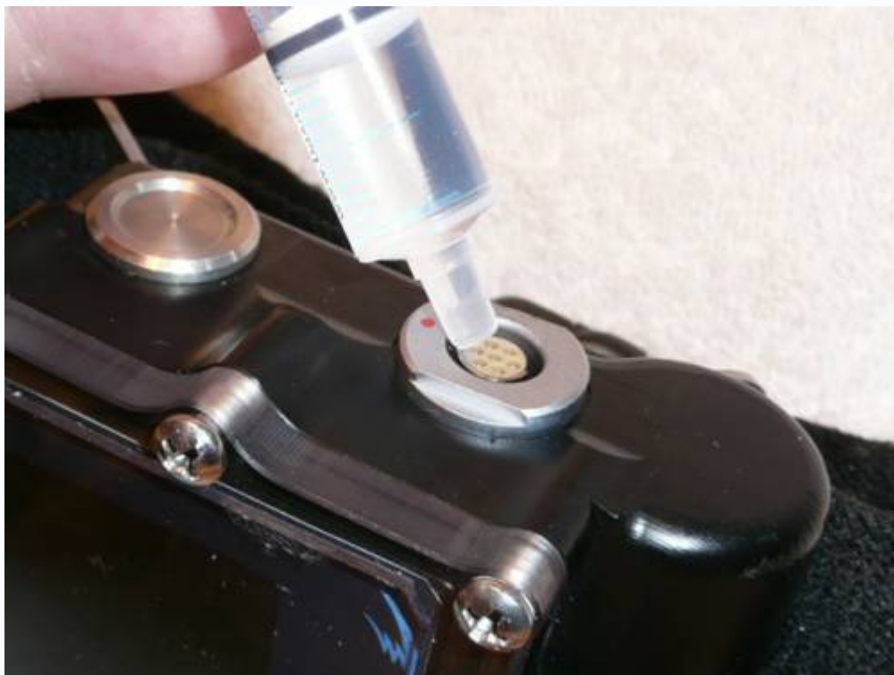
Adding Mineral Oil to Fischer Socket
