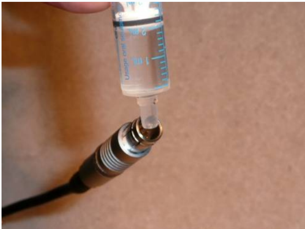
Drying Female Fischer Socket
