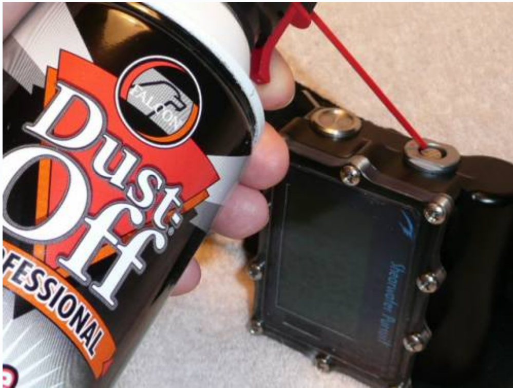
Adding Mineral Oil to Fischer Socket
